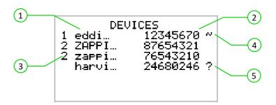
All linked devices (1) are listed in the DEVICES screen, the device shown in CAPITAL letters is the device currently being viewed. The serial number of each device is shown on the right (2)
