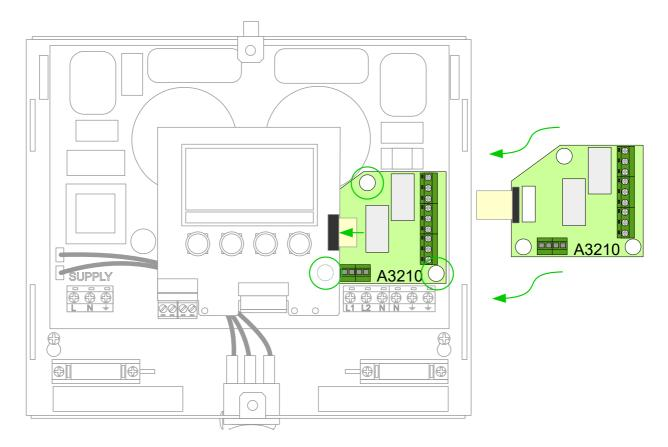
The Relay & Sensor Board is installed by plugging it into the **eddi** main circuit board using the three plastic spacers included with the Relay & Sensor Board.
