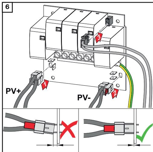
Connect the supplied cables to the respective connections on the PC board.
