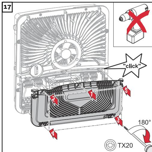
Place the cover on the connection area. Tighten the 5 screws by rotating them 180° to the right in the indicated order using a screwdriver (TX20).
