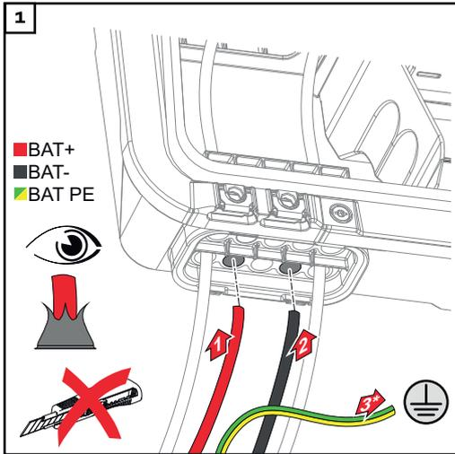
Manually push the battery cables through the DC bushings.
