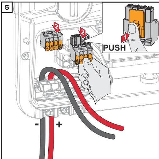
Press the lock on the back of the terminal and remove the DC terminals.
