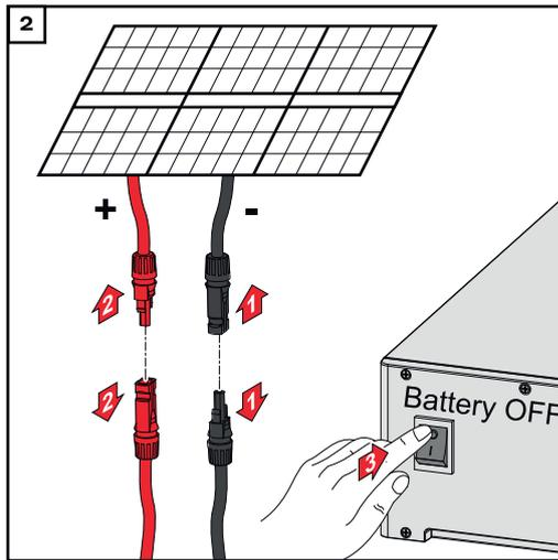
Disconnect connections from the solar module strings (+/-). Switch off the battery connected to the inverter.
