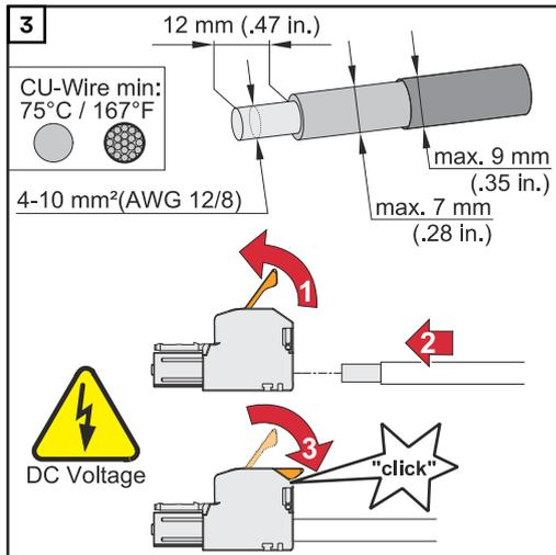
Select the cable cross section in accordance with the instructions in **Permissible cables for the electrical connection** from page 51.
