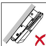
Do not install the inverter overhanging with the connection sockets at the bottom.
