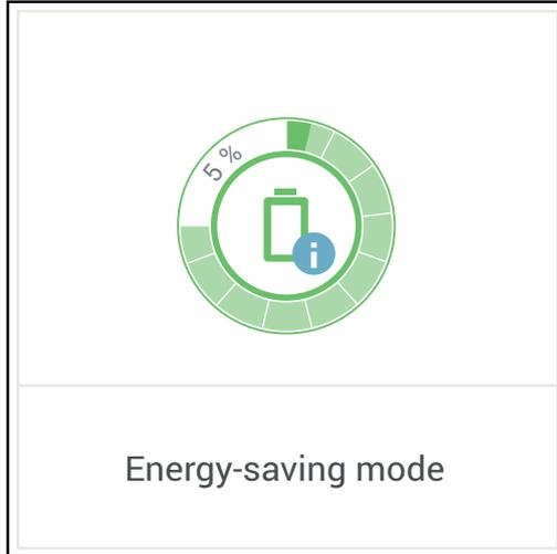
Energy saving mode is shown on the user interface of the inverter and in Solar.web by an "i" beside the battery symbol in the system overview.
