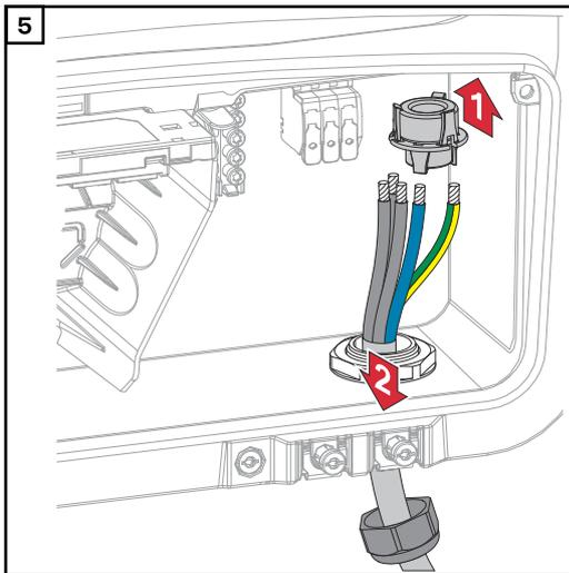
Take the ferrite core off and remove the mains cable from the inverter.
