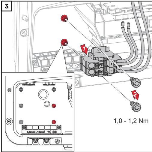
Insert the DC Connector GEN24 into the inverter and secure with the two screws (TX20) supplied at a torque of 1.0 - 1.2 Nm.
