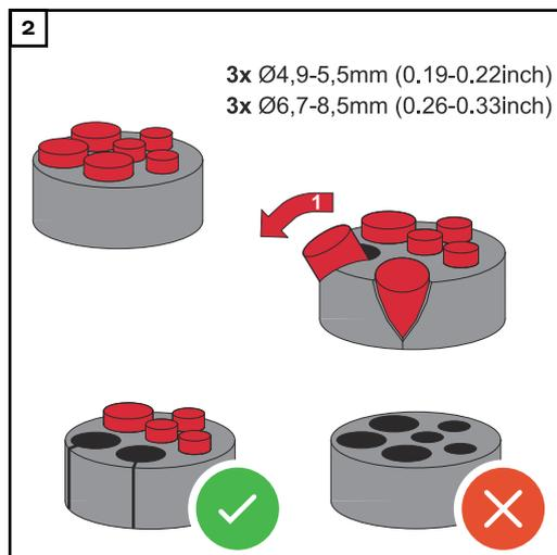
Open up the sealing ring at the location where the blanking plug is to be removed.
