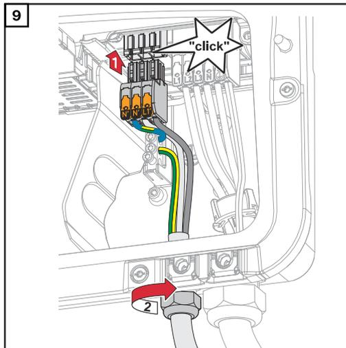
Insert the OP terminal into the OP slot until it engages. Tighten the union nut of the cable gland to the torque specified by the manufacturer.
