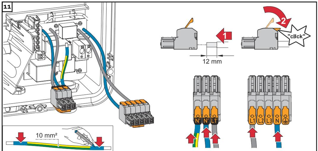
Strip the insulation of the single conductors by 12 mm. Lift to open the AC terminal's operating lever and insert the stripped single conductor into the slot provided, all the way up to the stop. Then close the operating lever until it engages.
