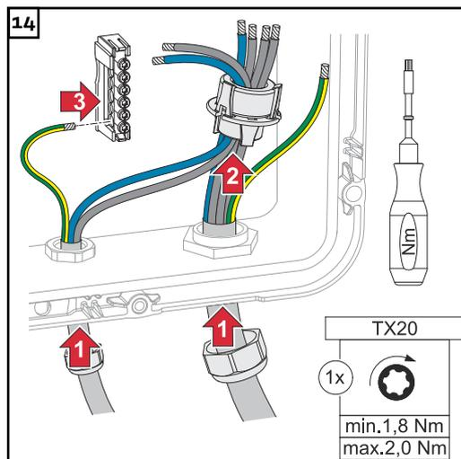
Route the phase/neutral conductors through the ferrite core. Fasten the ground conductor at the first input to the ground electrode terminal using a screwdriver (TX20) and a torque of 1.8-2 Nm.
