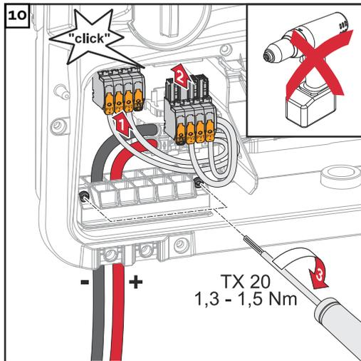
Insert the DC terminals into the respective slot until they engage. Fasten the screws of the strain-relief device to the housing using a screwdriver (TX20) and tighten to a torque of 1.3-1.5 Nm.
