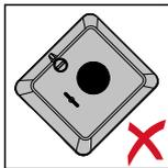
Do not install the inverter at an angle on a vertical wall or column.
