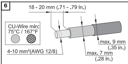
Strip the insulation of the single conductors by 18-20 mm. Select the cable cross section in accordance with the instructions in **Permissible cables for the electrical connection** from page 51.
