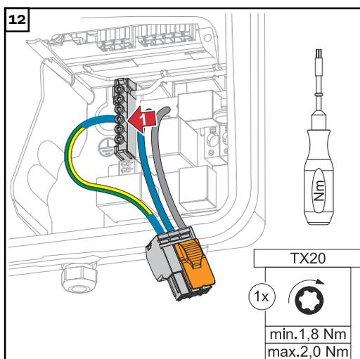
Fasten the PEN conductor to the third input of the ground electrode terminal from below using a screwdriver (TX20) and a torque of 1.8 – 2 Nm.
