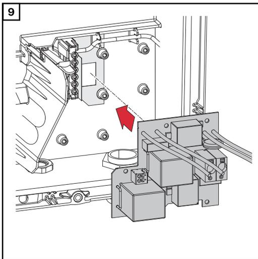
Install the PC board in the inverter.
