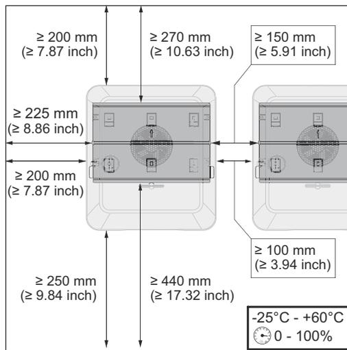
Only install on a solid, non-flammable surface.
