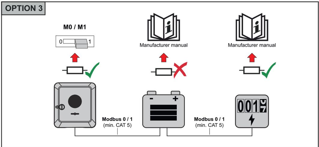
**Installing the WSD (wired shutdown)**
