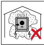
The inverter is designed to be dustproof (IP 66). In areas of high dust accumulation, dust deposits may collect on the cooling surfaces, and thus impair the thermal performance. Regular cleaning is required in this case, see chapter **Operation in dusty environments** on page 153. We therefore recommend not installing the device in areas and environments with high dust accumulation.
