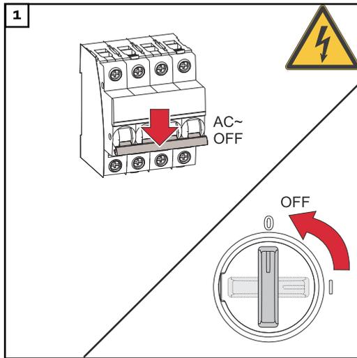
Switch off the automatic circuit breaker and DC disconnecter. Turn the DC disconnecter to the "Off" switch position.
