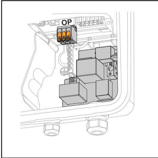
With PV Point Comfort, 1-phase electrical devices are continuously supplied up to a maximum power of 3 kW. Switching between grid-connected and backup power mode takes place automatically. In the event of a failure of the public grid or the inverter, the loads on the PV Point Comfort continue to be supplied. When the public grid is available again and stability is assured, the PV Point Comfort automatically switches to grid-connected operation and backup power mode is terminated.
