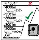
The inverter must not be installed or used at altitudes above 4000 m.
