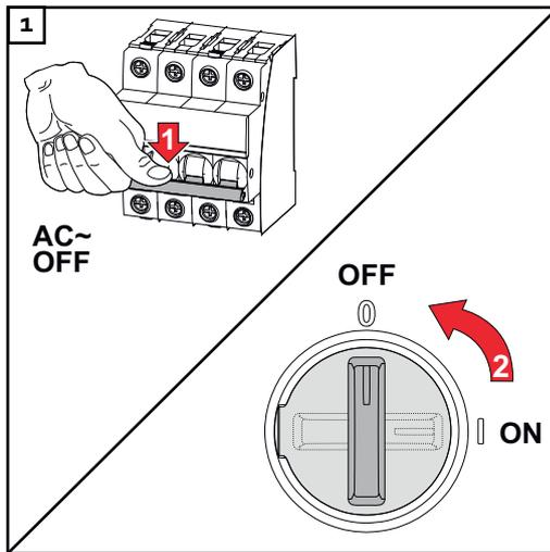
Turn off the automatic circuit breaker. Set the DC disconnect to the "Off" switch position.
