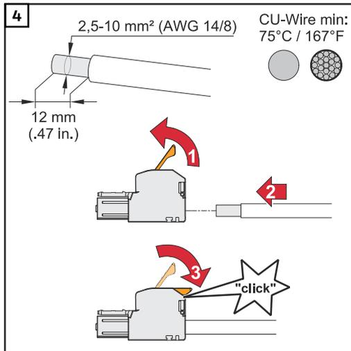
Strip the insulation of the single conductors by 12 mm. Select the cable cross section in accordance with the instructions in **Permissible cables for the electrical connection** on page 51. Lift to open the terminal's operating lever and insert the stripped single conductor into the slot provided as far as it will go. Then close the operating lever until it engages.
