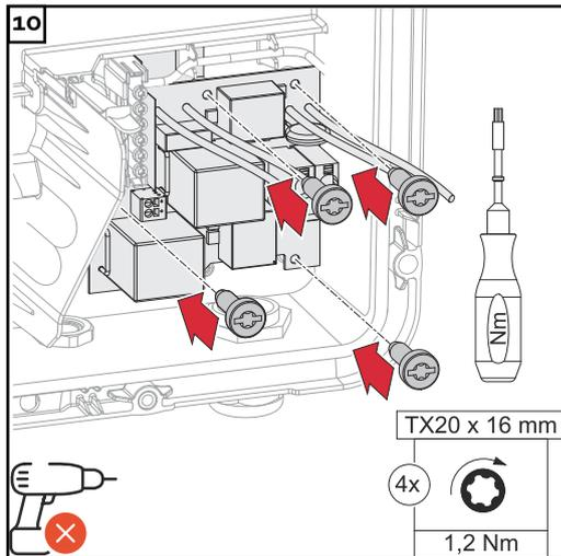
Fasten the PC board with the 4 screws (TX20) supplied and tighten to a torque of 1.2 Nm.
