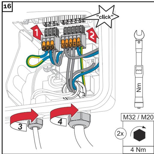
Insert the terminals into the respective slot until they engage. Tighten the union nut of the cable gland to a torque of 4 Nm.
