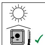
The inverter should be installed in a protected location, for example, below the PV modules or under an overhanging roof.
