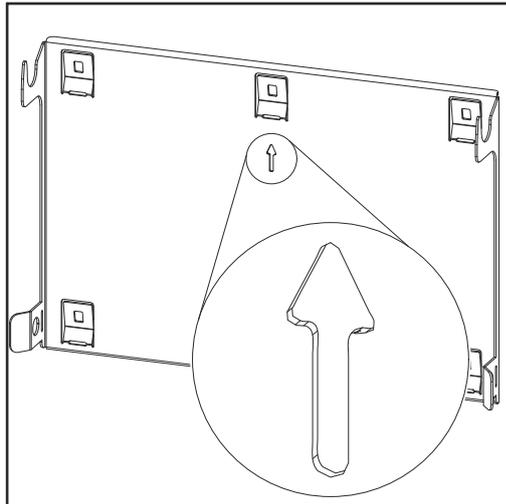
The mounting bracket (illustration) is also used as the gauge.
