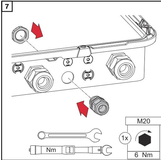
Insert the cable gland into the bore and tighten to a torque of 6 Nm.
