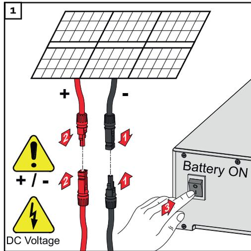
Connect the solar module strings (+/-). Switch on the battery connected to the inverter.
