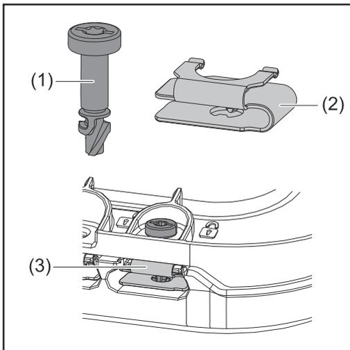
A quick-lock system (3) is used to mount the connection area cover and front cover. The system is opened and closed with a half-rotation (180°) of the captive screw (1) into the quick-lock spring (2).
