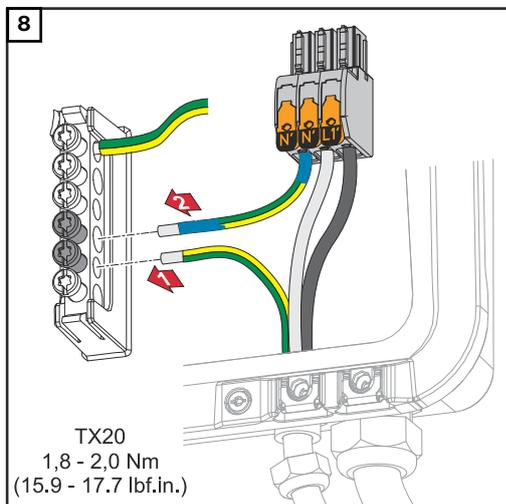
Fasten the ground conductor and PEN conductor to the ground electrode terminal using a screwdriver (TX20) and tighten to a torque of 1.8-2 Nm.
