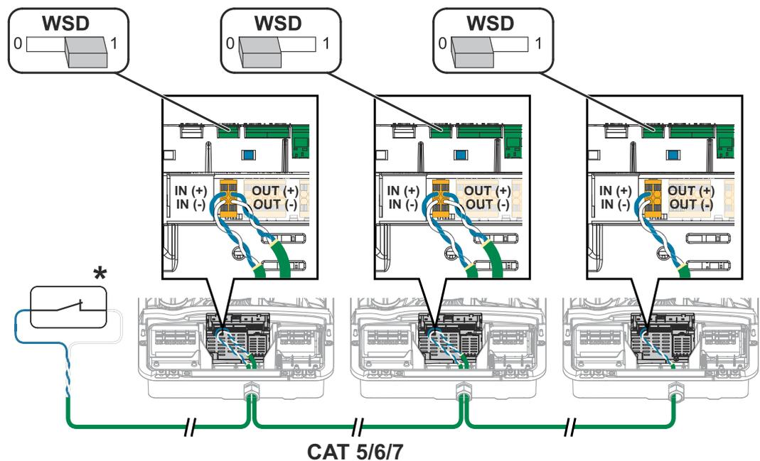
\* Floating contact of the trigger device (e.g. central grid and system protection). If several floating contacts are used in a WSD chain, they must be connected in series.
