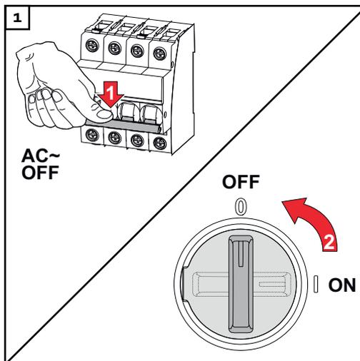
Turn off the automatic circuit breaker. Set the DC disconnecter to the "Off" switch position.
