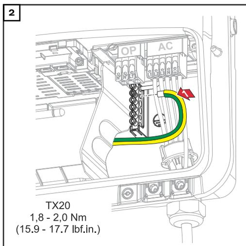
Fasten the battery ground conductor to the second input of the ground electrode terminal from the top using a screwdriver (TX20) and a torque of 1.8 – 2 Nm.
