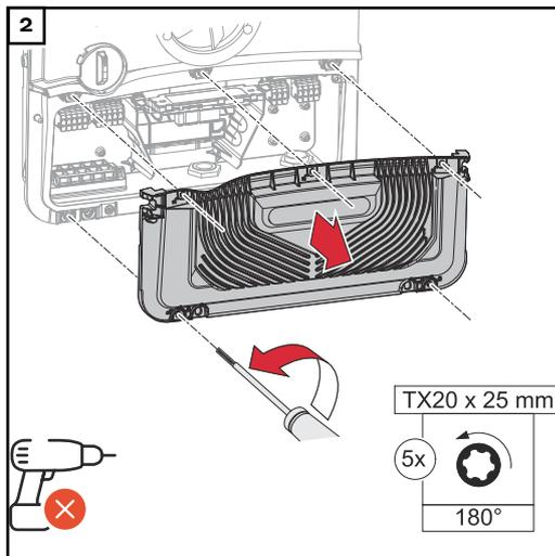
Loosen the 5 screws of the connection area cover by rotating them 180° to the left using a screwdriver (TX20). Remove the connection area cover from the device.
