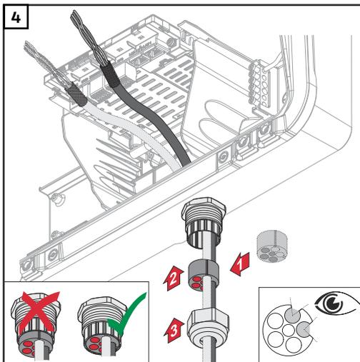
Insert the sealing ring between the union nut and the housing opening. Press the data cables into the seal's cable guide. Then press in the seal until it reaches the underside of the cable gland.
