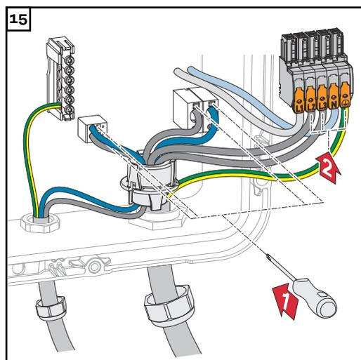
Connect the stripped phase/neutral conductors to the terminals provided.
