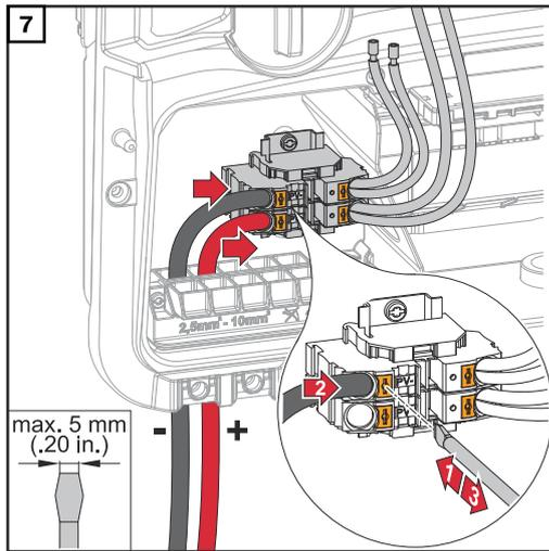
Use a slotted screwdriver to push in the lock on the terminal. Insert the stripped single conductor into the slot provided, in each case as far as it will go. Then withdraw the slotted screwdriver from the lock.
