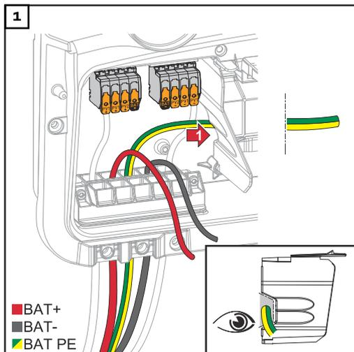
Route the battery ground conductor into the integrated cable duct of the connection area divider and into the AC connection area.
