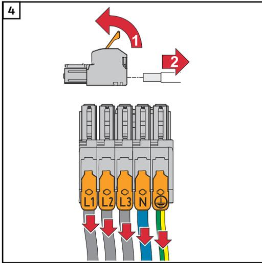
Disconnect the individual conductors from the AC terminal (only necessary if the installation already exists).
