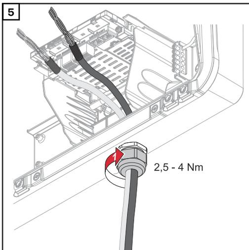
Tighten the union nut for the cable gland to a torque of min. 2.5 to max. 4 Nm.
