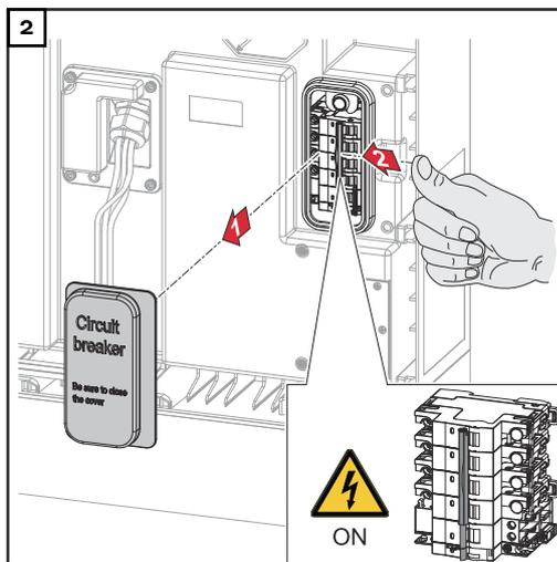
Pull off the cover of the DC disconnect to the front. Set the DC disconnect to the "On" switch position.
