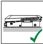
The inverter is suitable for a horizontal installation position.
