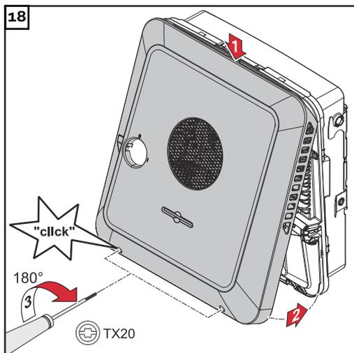
Clip the housing cover onto the inverter from above. Press on the lower part of the housing cover and tighten the 2 screws by rotating them 180° to the right using a screwdriver (TX20).
