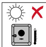
In order to minimise the heating up of the inverter, do not expose it to direct insolation.
