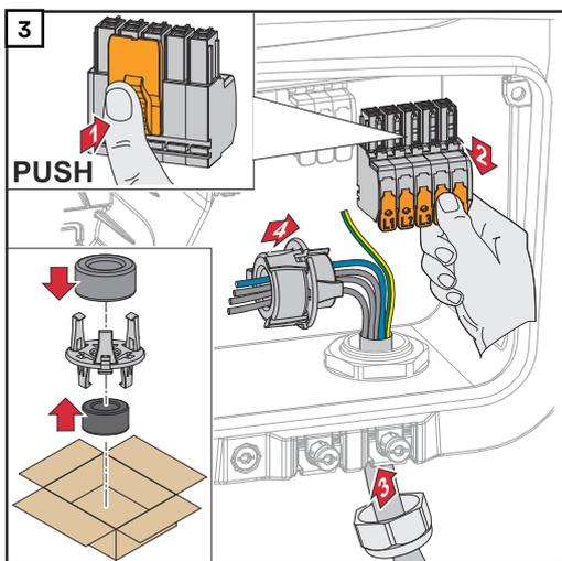
Press the lock on the back of the terminal and remove the AC terminal. Route the mains cable from below through the cable gland on the right side and the ferrite core.
