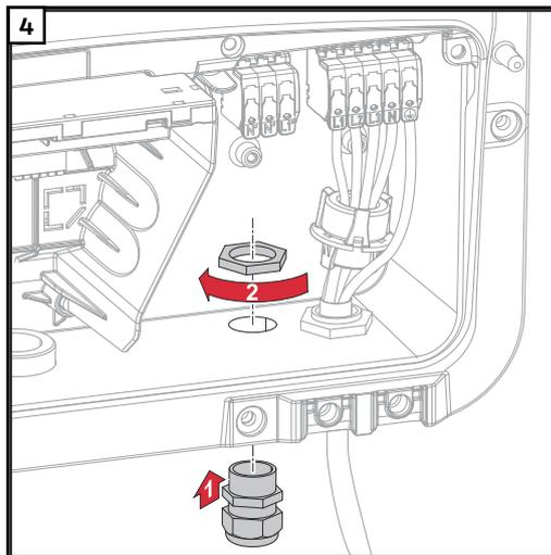
Insert the cable gland into the bore and secure to the torque specified by the manufacturer.
