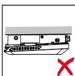
Do not install the inverter on the ceiling.
