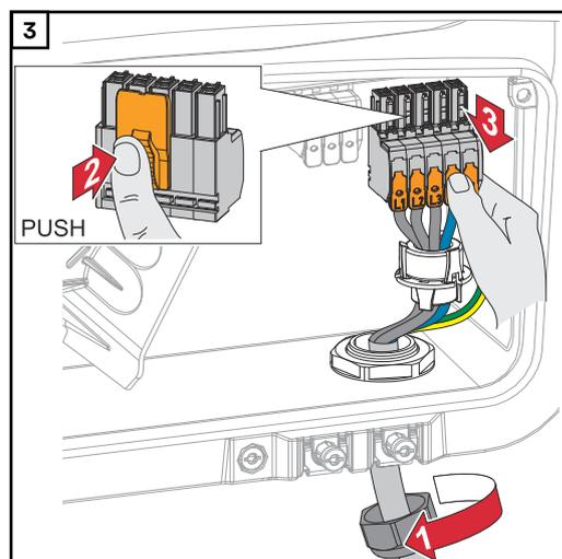
Press the lock on the back of the terminal and remove the AC terminals. Undo the cable gland.
