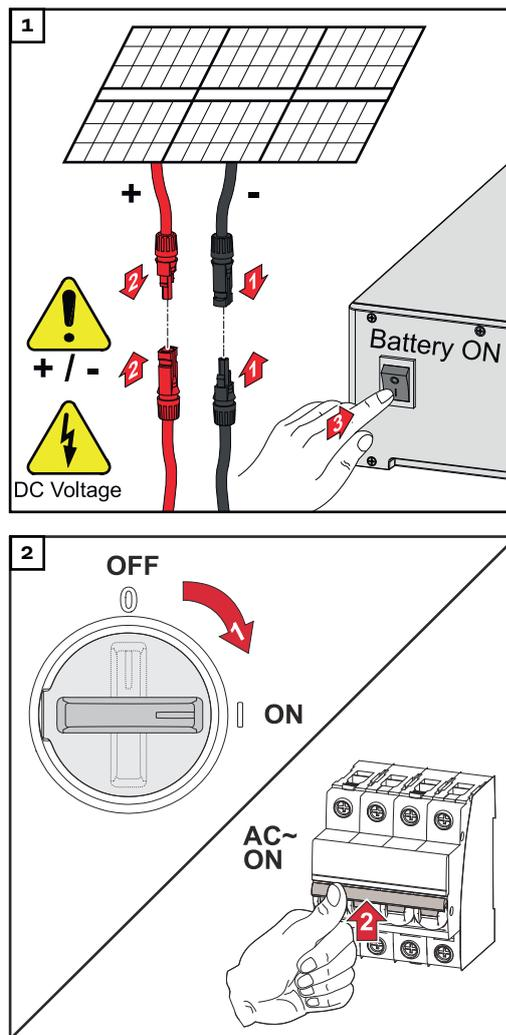
Connect the solar module strings (+/-). Switch on the battery connected to the inverter.
