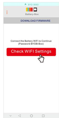
4. After downloading the firmware, tap the button "Check WIFI Settings" to connect the Wi-Fi of the battery, which begins with "BYD-", and the full name could be found at BMU. All the Wi-Fi shares the common password (BYDB-Box).
