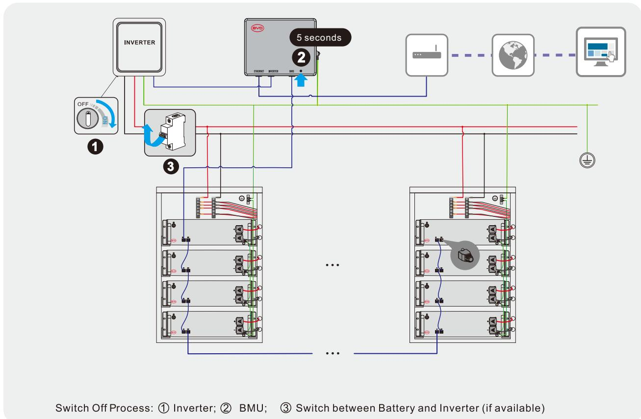
Switch Off Process: ① Inverter; ② BMU; ③ Switch between Battery and Inverter (if available)
