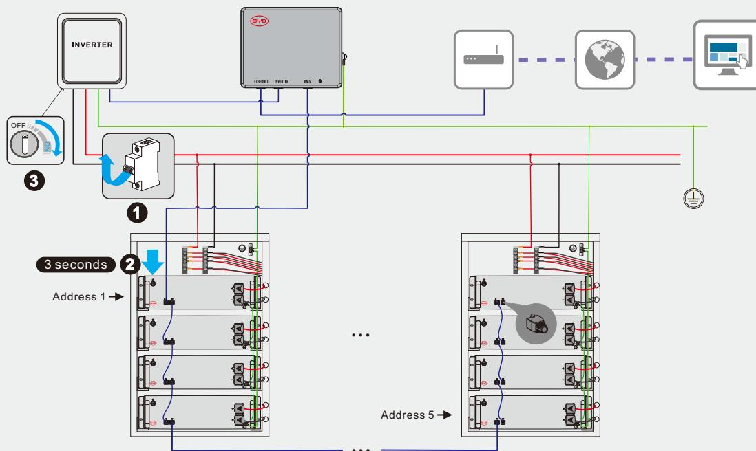
Switch On Process: ① Switch between Battery and Inverter (if available); ② Battery; ③ Inverter
